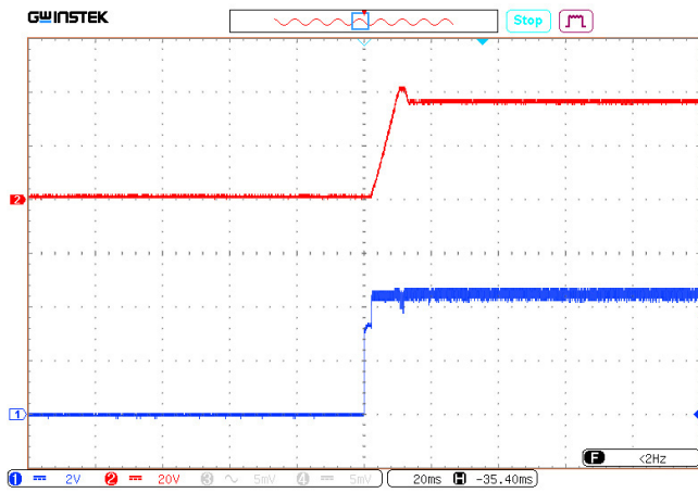
Figure 24. U_{OUT,NOM} stabilizing with Remote On/Off option (ON and -OUT pins connection).
