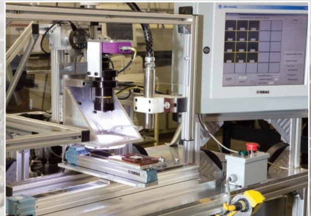
Automated optical inspection improves accuracy and provides the stringent level of quality control required in high reliability applications.
