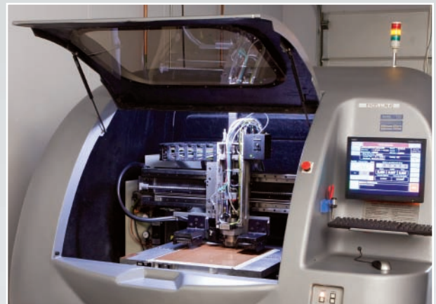
Precision drilling and routing equipment allows fast turnaround on prototypes and endless customization capability.
